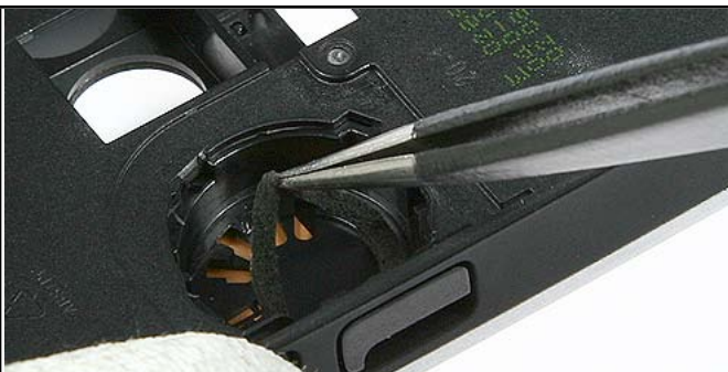
18.) Always remove the residues of the IHF Gasket. Use a new one when reassemble.
