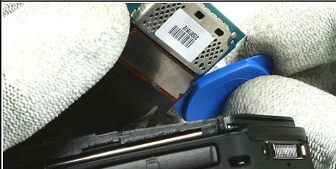
13.) Carefully release the flex connector at one side first.
