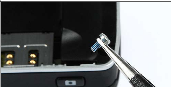
4.) Once removed, the screws can't be used again. Always use new screws for assembly.
