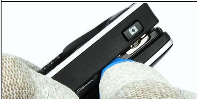
5.) Release the clips of the D-Cover.
