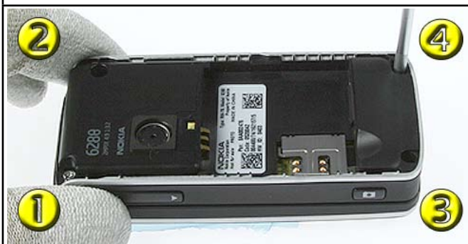
3.) Unscrew all Torx size 6 plus screws in the shown order. For Assembly use the reverse order and a torque of 25 Ncm.
