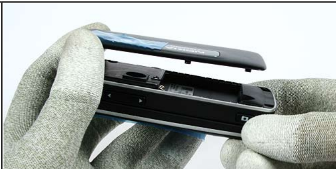
2.) Ensure that no battery is inserted.
