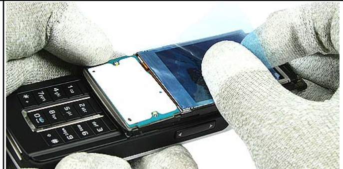
10.) Protect the LCD with a plastic film.
